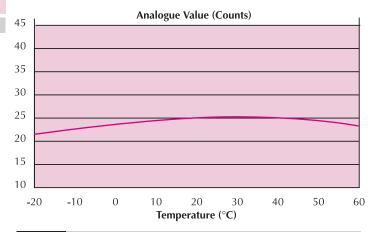
Typical Temperature Response - XP95 Optical Smoke Detector
